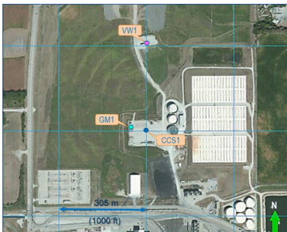
Figure C.9. Map of well locations (below) and diagram (right) for vertical arrays showing configuration of borehole and monitoring equipment for the IBDP site in relation to stratigraphy: the WellWatcher PS3 geophone array in the CCS1 well; the OYO, three-component, 31-level array in the GM1 well; and the Westbay system in the VW1 well for sampling and pressures readings at 11 levels. Source: from Will et al. 2014.
